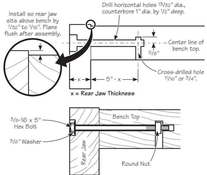
The horizontal holes should first be drilled 13/32" dia. through the rear jaw. Then, with the rear jaw 1/32" to 1/16" proud of your bench top, transfer these holes and continue drilling them 35/8" to 4" deep. The intersecting cross-drilled holes should now be drilled. To ensure that the cross-drilled holes intersect with the horizontal holes, a simple alignment tool can be made from 3/8" dowel, a block of scrap, and a nail.
