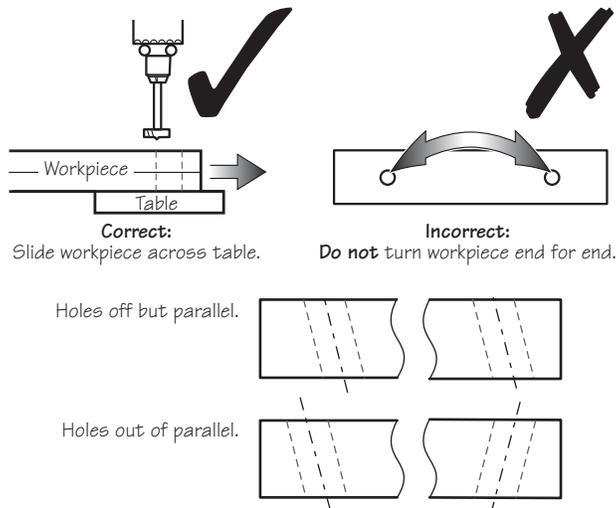
6. You need to drill two holes in the rear jaw for the steel dowel pins, which will keep your work off the vise screws, and two corresponding clearance holes in the front jaw. All four holes are drilled in the **inside faces** of the front and rear jaws. Lay out the holes as follows and drill the holes for the rear jaw  $\frac{3}{8}$ " dia. by 1" deep and the ones for the front jaw  $\frac{1}{2}$ " dia. by  $\frac{15}{8}$ " deep.
