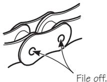
Assemble the spring-clip-type connecting link as per diagram:
