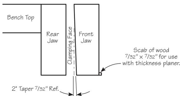
8. Insert the vise screw nuts into the back of the rear jaw, aligning them square. Using a  $\frac{1}{4}$ " drill bit in the screw holes, lightly mark the centers. Before removing the nuts, mark both the orientation for realignment and the hole each came from. Remove
