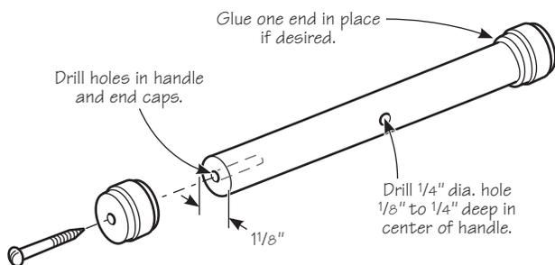
To assemble the speed knob, take one of your handles (right side if you are right handed) and drill a  $\frac{17}{64}$ " hole through the center (see illustration at right).
