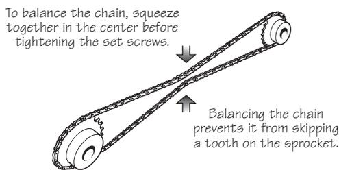
If after installing your chain you observe any sag, use one or two of the #10 wood screws and chain rollers to support the bottom of the chain. **Do not** install the spacer any higher than the bottom of the chain loop when taut.
