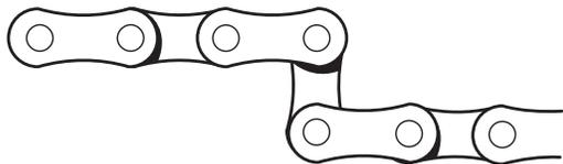
If this is the case, to remove half of a link you must first remove a full link (as shown on page 3) then add the half link supplied. The half link is assembled in the same manner as the full link (and must be installed next to the full link). To lock the half link, insert the pin, then slide the cotter pin through the small hole and spread open the cotter pin (see illustration).
